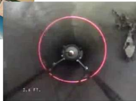
Laser Ring Profiler: Deflection Measurement
